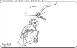
Squeeze and hold trigger to release cleaning solution (Fig.5/6). Push cleaner forward SLOWLY then pull it back SLOWLY.
